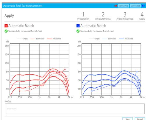
Once saved, you can view the results for the REUG, REOG, Acoustic Coupling and Aided Measurements on the Fitting > Automatic REM screen.
